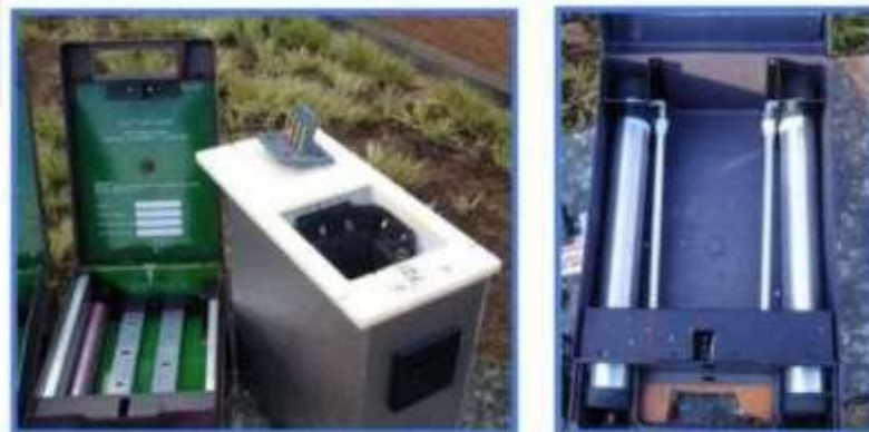
TYPICAL CIT APPLICATION SHOWING DYE DISCHARGE TUBES
